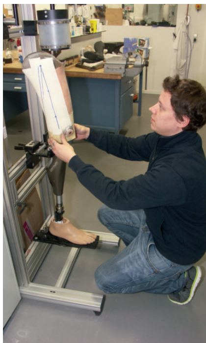
Fitting the shaft to a high-tech prosthesis.
